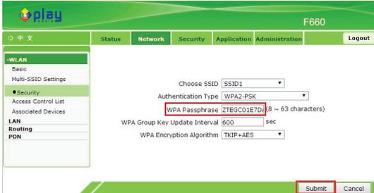
The screenshot shows the 'Security' tab of the play F660 web interface. The 'WLAN' section is expanded to 'Security'. The 'WPA Passphrase' field is highlighted with a red box. The 'Submit' button at the bottom right is also highlighted with a red box.
